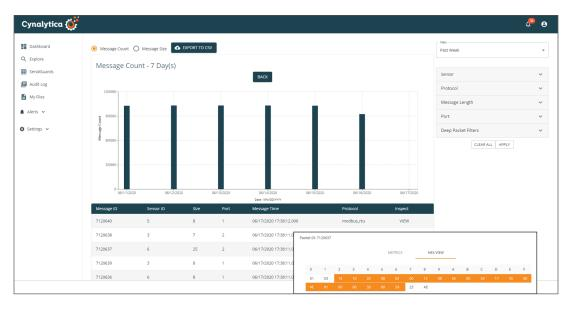
AnalytICS Engine, SerialGuard's supporting platform, operates as an intrusion detection system (IDS) and data analytics tool. The software offers operators the ability to securely capture, baseline and analyze trends in serial communications through encrypted communications.
